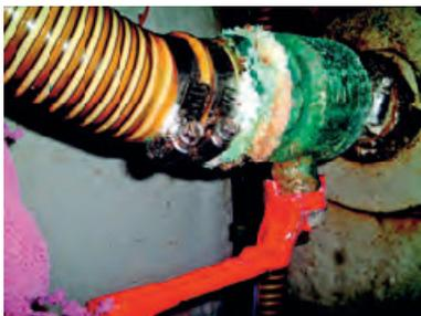
*Most modern boats have ball valves. This one needs replacing*
