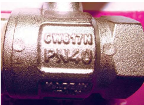
Brass valve removed from packaging and turned over to show marking
