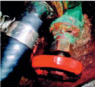
*Many used boats have gate valves. This one is terminally corroded*
